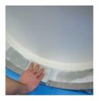
Lightly dab sponge along the water soluble tape portion of the dam to increase dam adhesion and ensure zero air permeability.
