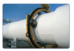
TAG also manufactures heavier duty steel construction split frame cutting and bevelling machines. Rugged in design, and built to stand up to the most arduous of site conditions.
