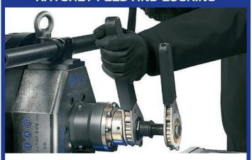
The PREP 16 has unrivalled power and stability, utilising a ratchet system for both jaw locking, and bevel feed.
